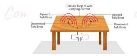
For the downward direction of the current, the direction of the magnetic field will be as if emerging from the table outside the loop and merging the table inside the loop. Similarly, for current flowing in the upward direction, the direction of the magnetic field will as if they are emerging from the table outside the loop and merging to the table inside the loop as shown in the figure.
