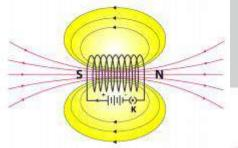
When the north pole of the bar magnet is brought close to the end connected to the negative terminal of the battery, the solenoid repels the battery. As like poles repel each other, we can infer that the end connected to the negative terminal behaves as a north pole while the end connected to the positive terminal behaves as a south pole.
