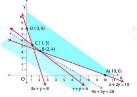
A (10, 0), B (2, 4), C (1, 5) and D (0, 8) are the corner points of the feasible region. The values of z at these corner points are given below
