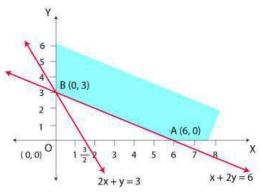
A (6, 0) and B (0, 3) are the corner points of the feasible region. The values of Z at the corner points are given below
