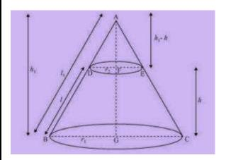
Let ABC be a cone. From the cone the frustum DECB is cut by a plane parallel to its base. Here, r<sub>1</sub> and r<sub>2</sub> are the ready of the frustum ends of the cone and h be the frustum height. Now, consider the  $\triangle$ ABG and  $\triangle$ ADF,
