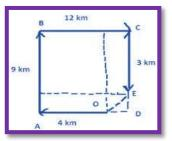
From the figure, the distance OE is to be calculated. In triangle ODE,  $OE = \sqrt{OD^2} + (DE^2)$ =  $\sqrt{(BC - AO)^2 + (AB - CE)^2} OE = \sqrt{(8^2 + 6^2)} = 10$ km.
